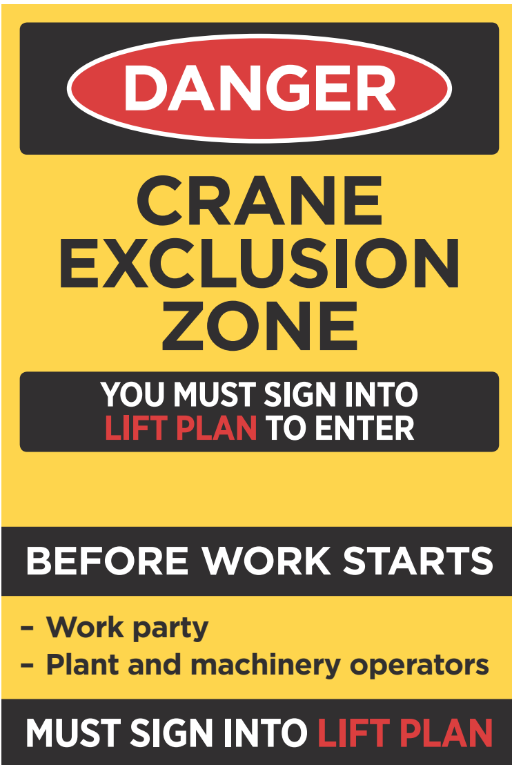
FIGURE 28: Crane exclusion zone 'sandwich board'
